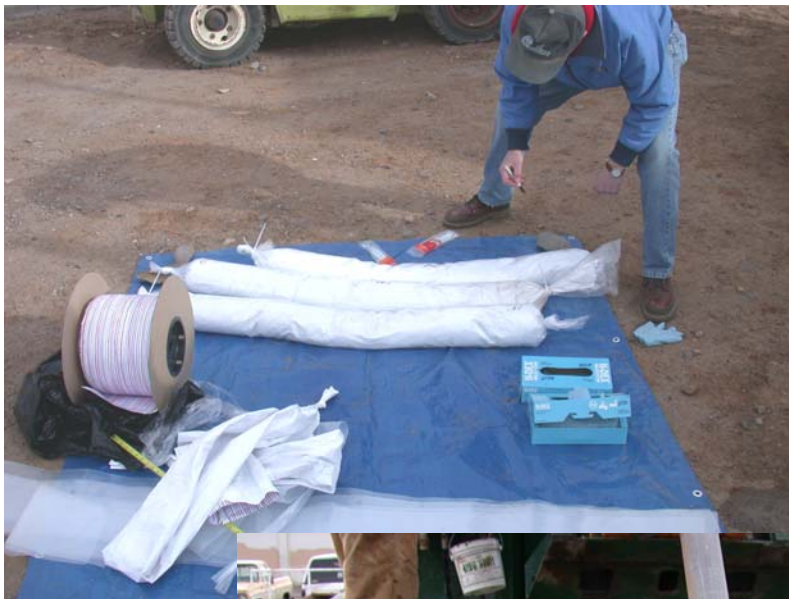
NAPL cover on reel and inverted with knot in end.
