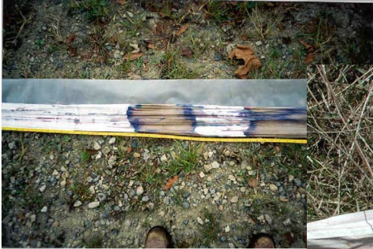
Bleeding fracture stains from core hole
