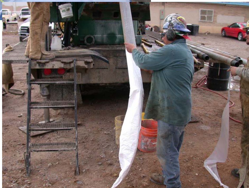
Sliding the NAPL FLUTE cover over the core barrel
