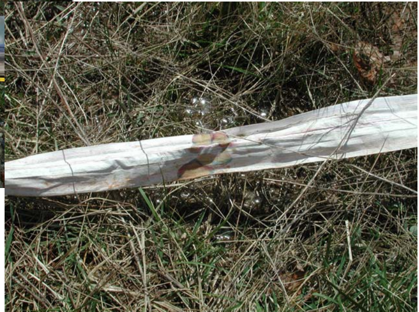
Bleeding fracture stains from core hole
