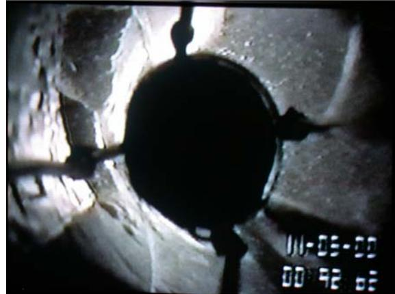
**Fig. 9. Interior view of liner conforming to hole**
